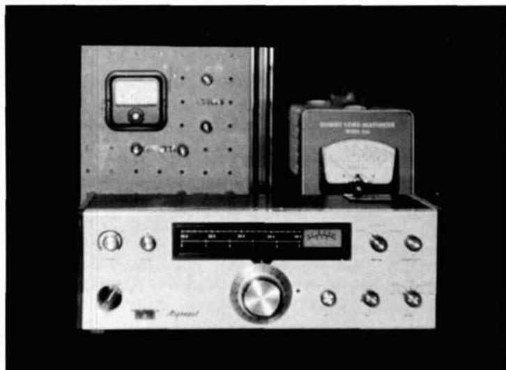
fig. 2. Basic solar-powered QRP station used by W3FQJ uses Ten-Tec Argonaut transceiver, solar power converter ( fig. 1 ), solar control panel ( fig. 4 ) and 12-volt motorcycle battery.
